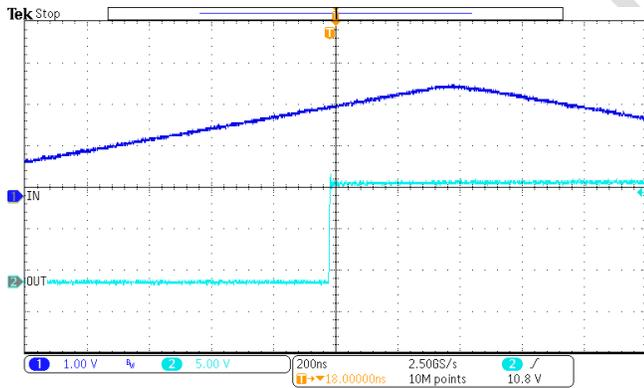
Figure 4. Driver Switching ON
